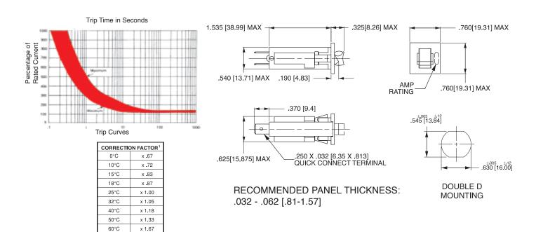
1. To adjust the breaker rating for ambient temperature, multiply the breaker rating by the factor. (ex: 5A rating x .850 = 4.25A. Select 4A rating.)
